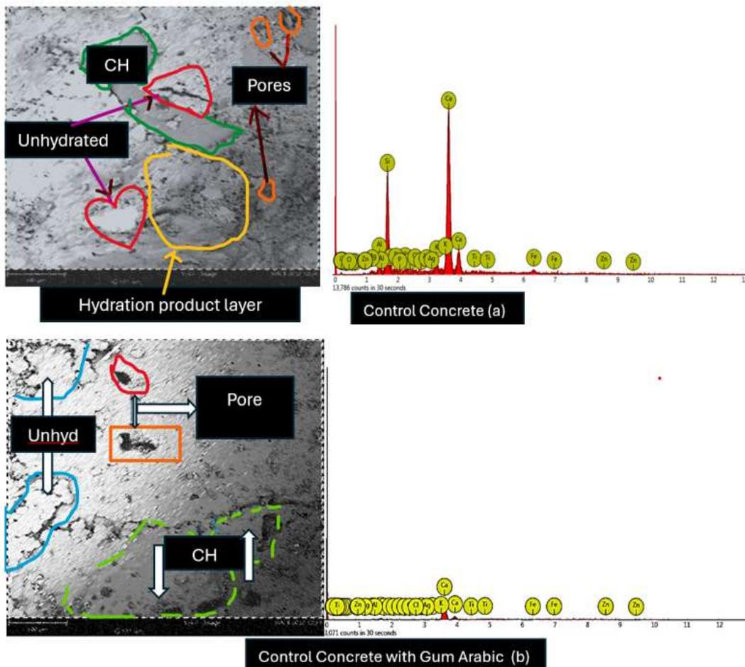
**Fig. 1: Micrograph and EDS Spectrum - Control Concrete (a): Control-GA Concrete (b)**
