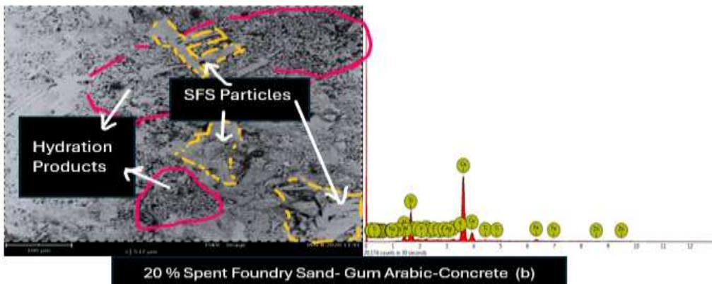
Fig. 3: Micrograph and EDS Spectrum of 20 % SFS-GA Concrete
