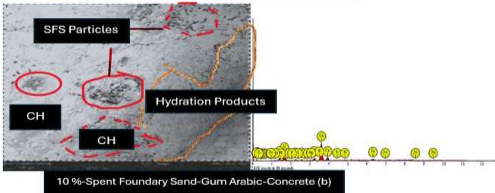
Fig. 2: Micrograph and EDS Spectrum -10 % SFS-GA Concrete
