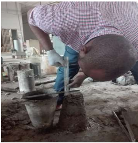
Plate 2: Slump test on fresh concrete.
