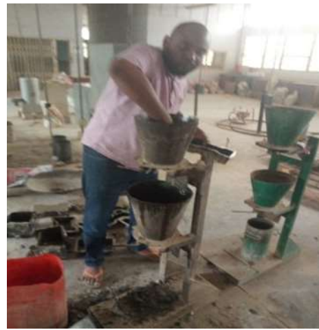
Plate 3: Compacting factor test
