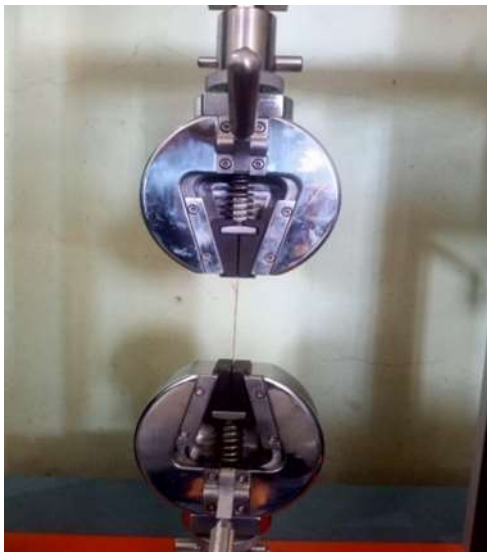
Plate 1. Fibre is ready for test in the machine
