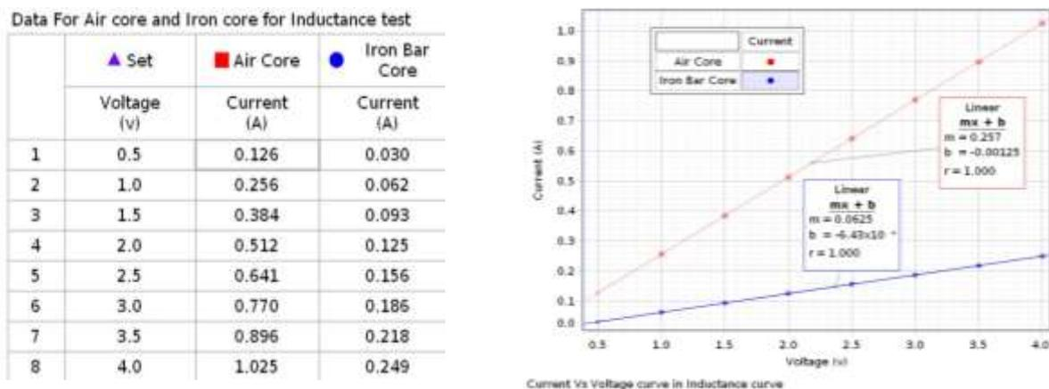
Fig 2. Inductance results for air sample and Iron bar baseline
