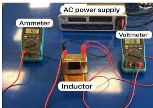
**Fig 2. Inductance test set up**
