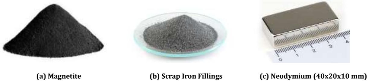
**Fig 1. Materials Used in Cement Mixtures**
