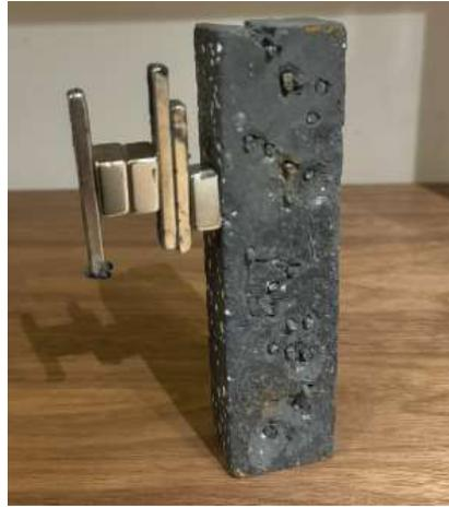
Fig 4. Modified cement mortar with enhanced magnetic properties
