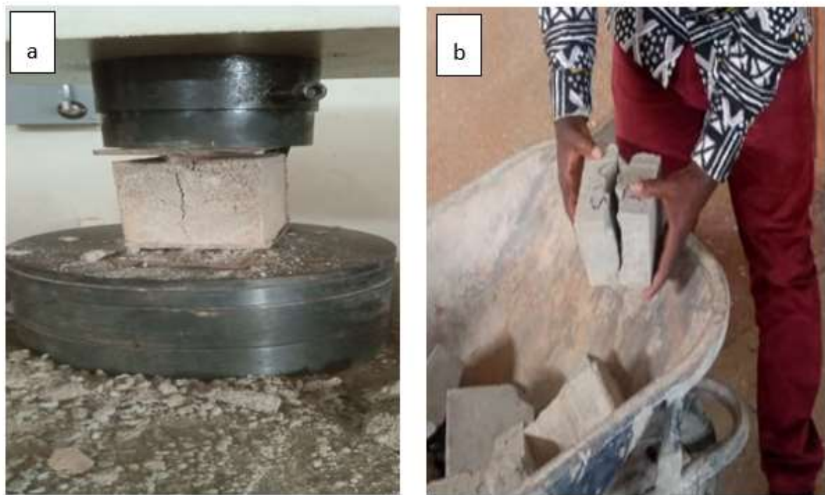
Fig 8 (a). Split tensile strength test, (b). Failure mode of the specimen.
