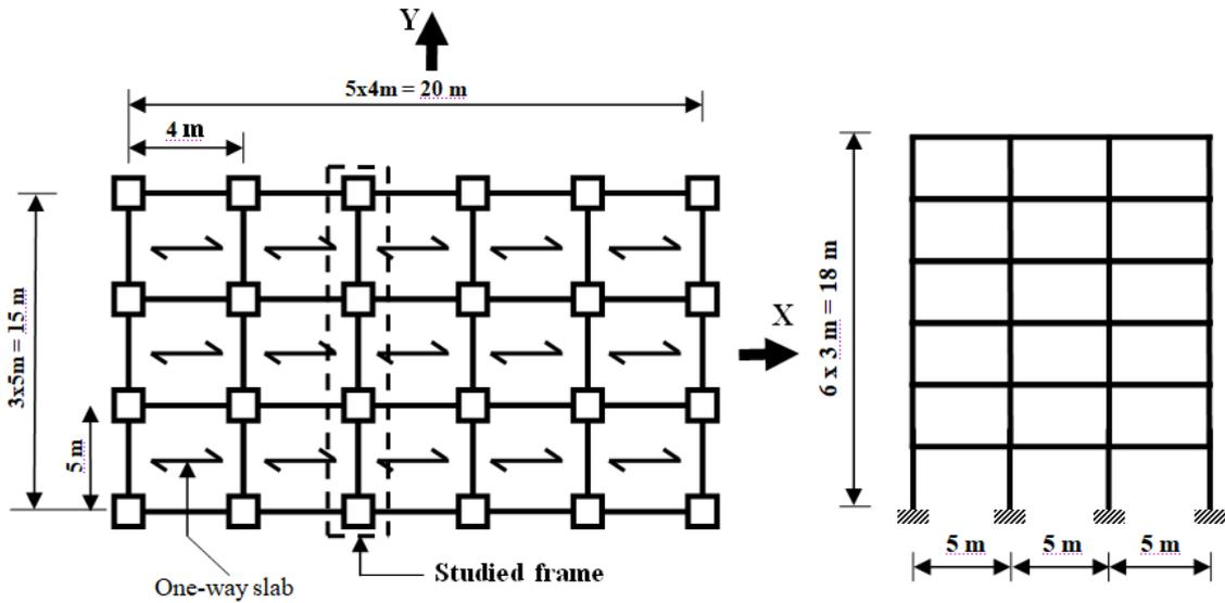
Fig 1. Plan view of the building and the studied frame.
