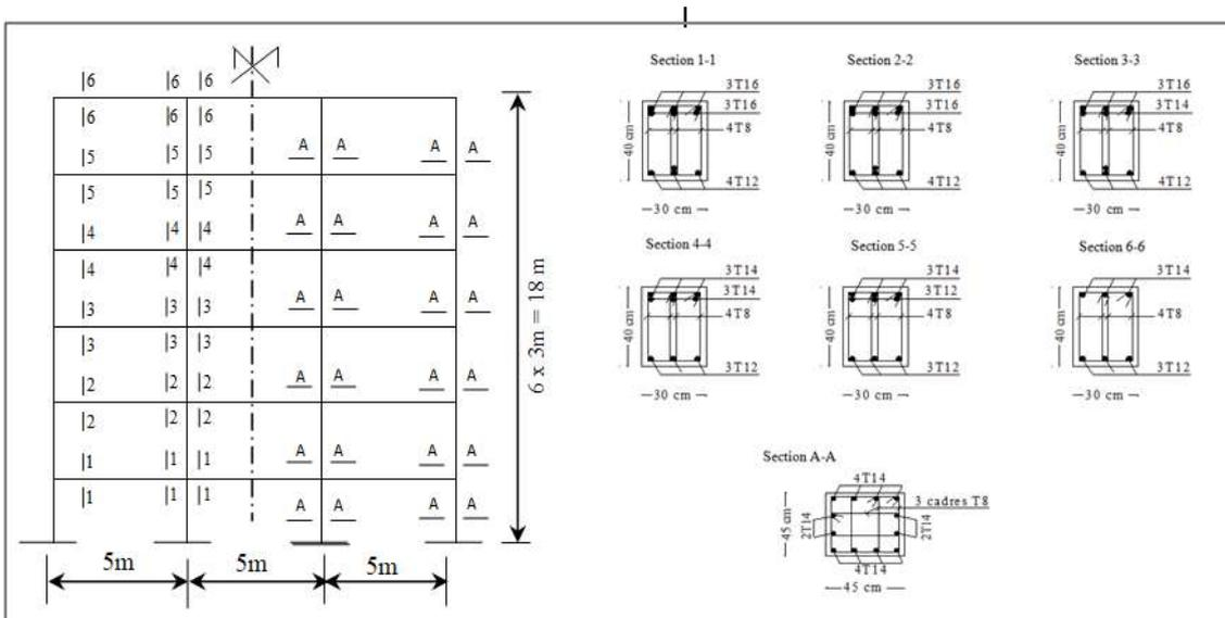
Fig 2. Dimensions and reinforcement details at both ends of the beams and the columns in the frame.
