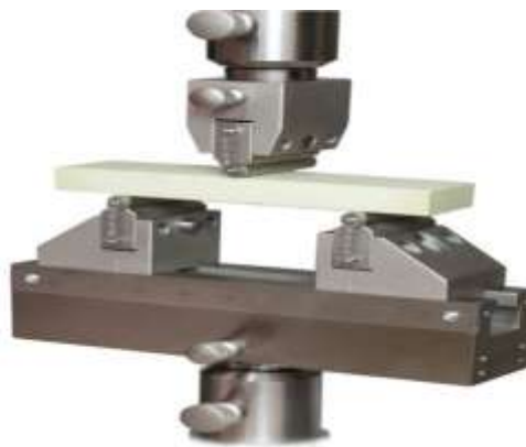
Plate 1: Standard set up of specimen on a UTM machine.
