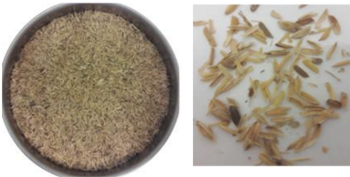
Fig.1. : Boat-like shape of the as received whole rice husk.
