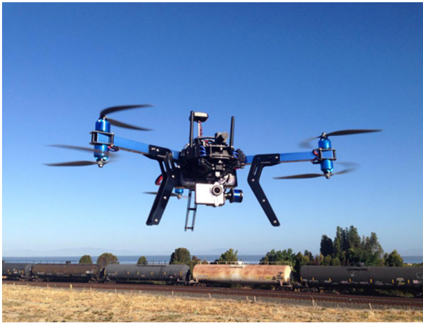
Figure 1: 3D Robotics Y6 hexacopter used as the reference UAV platform, adapted from Foster [8].
