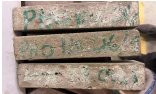
Fig. 5. Phosphate reaction with Cement Paste
