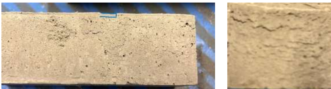
Fig. 4. Evidence of Swelling
