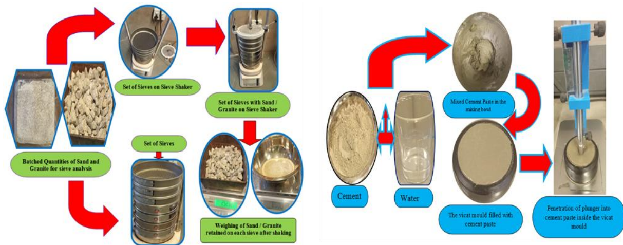
Fig. 1. (a) steps of determining the sand and granite particles' sizes through Sieve analysis (b) steps of determining the Consistency of Cement Paste
