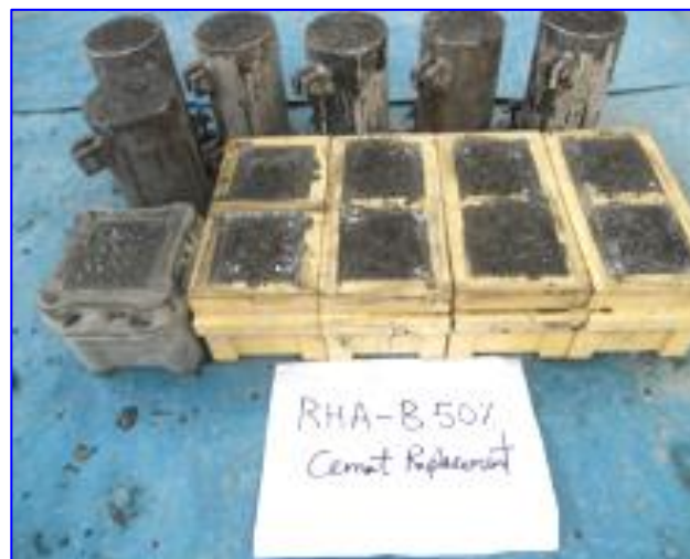
Fig 1. Casting of cubes and cylinders for compressive and splitting tensile strength of concrete, compressive and splitting tensile strength test according to BS EN 12390-3:2009.
