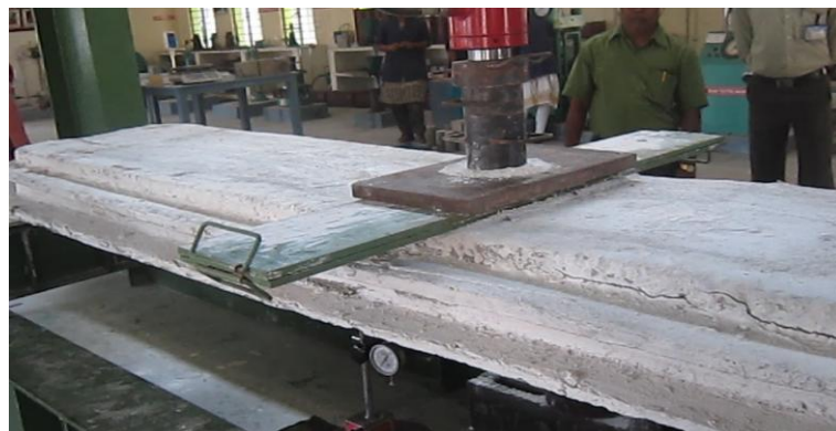
Fig. 5. Loading arrangement of the deck in the frame.
